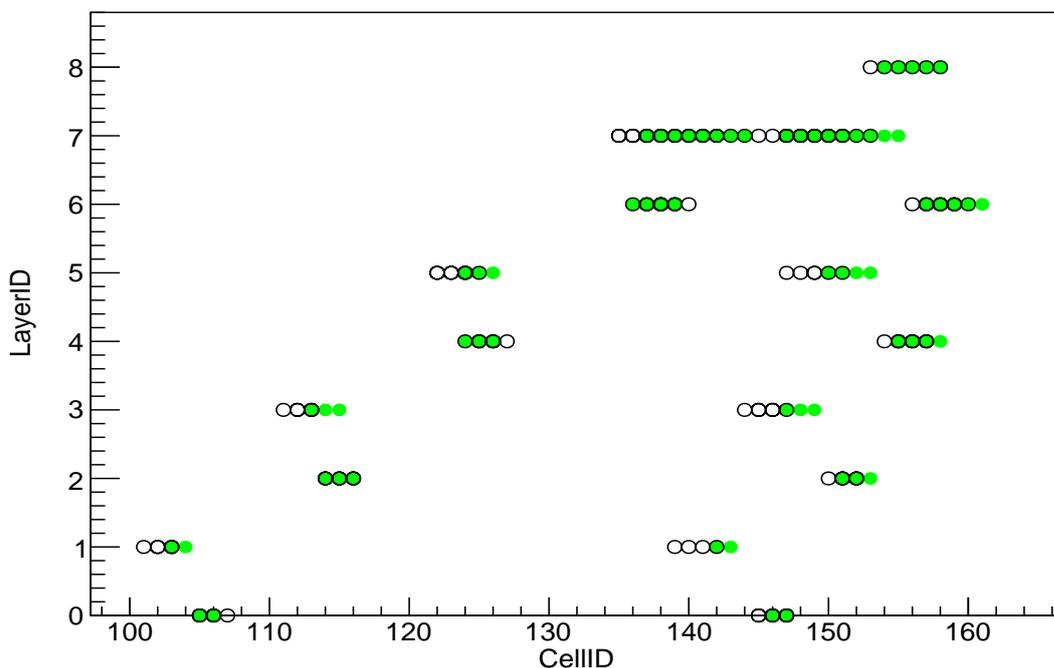
Figure 1: The incident hits of Event 24 clearly exhibits a feature of the first pattern, which has all the first turn hits at the right most of every layer. In terms of wire ID, for pattern 1, all the first turn hits have the largest wire ID within each layer.
