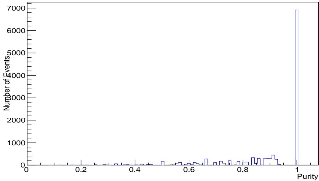
Figure 7: The maximum purity out of the four patterns identified for the outgoing hits. Only showed the distribution of events with more than 2 turns (chosen by `cdc_turnId`).
