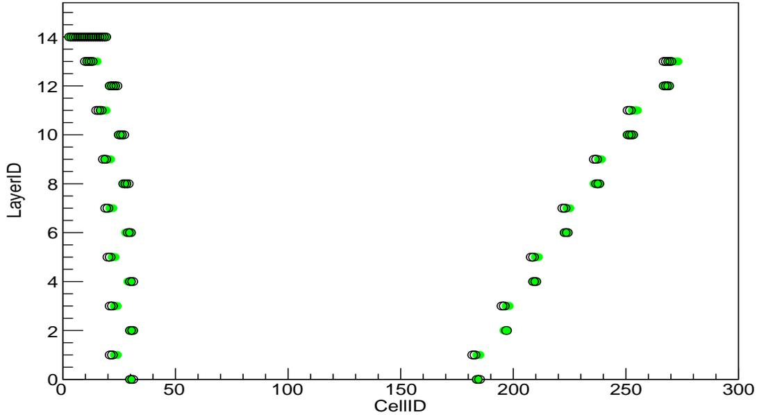
Figure 4: Event 82 has a clear feature which is classified as the special scenario. The trajectory enters the Cylindrical Drift Chamber from a special position such that the recorded wire ID for the incident hits are smaller than that of the exit ones.
