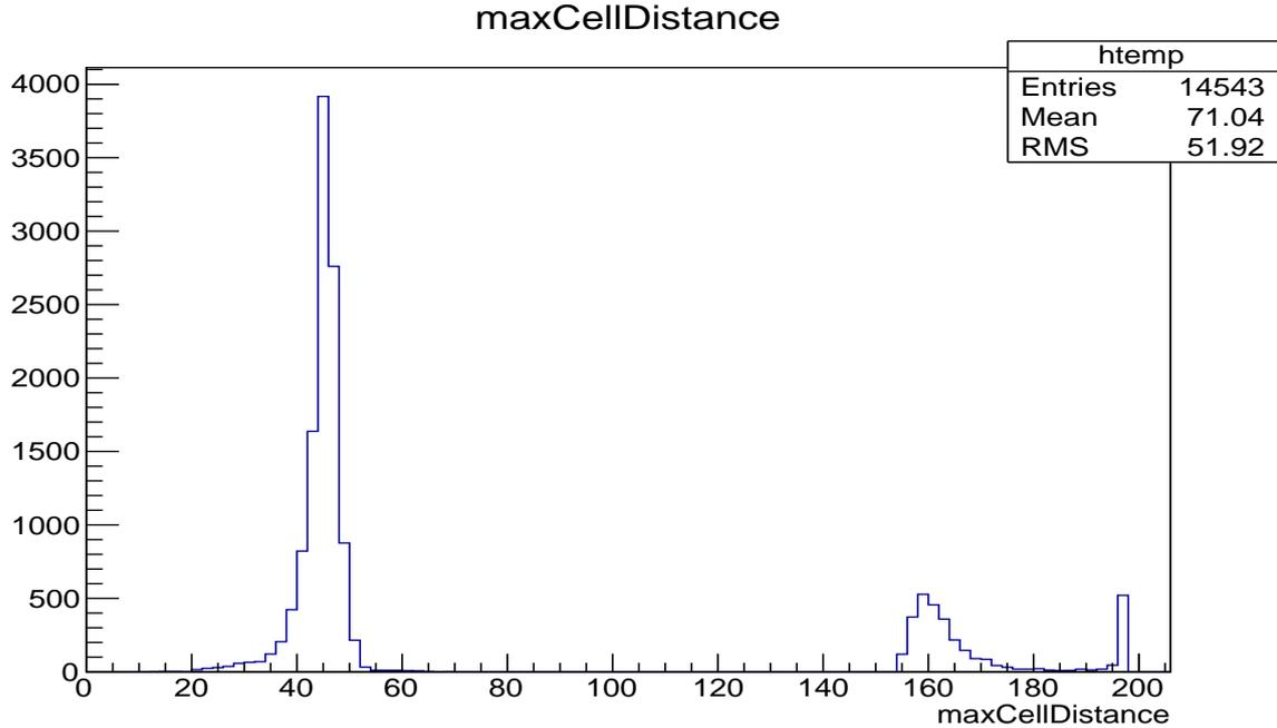
Figure 5: The distribution of maximum distance between the left most and right most hits' wire ID.
