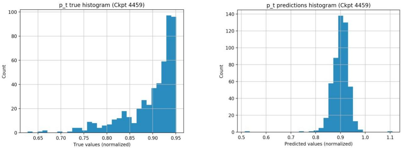
Figure 4: a) Example distribution of true tangential momentum values, clearly left-skewed. b) Corresponding predicted distribution from a trained deep neural network, clearly Gaussian in shape.
