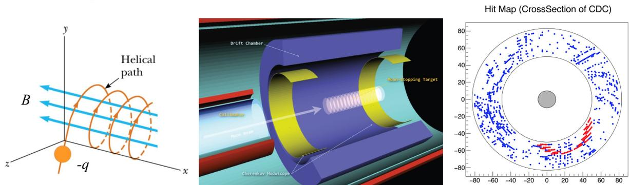
Figure 2: a) Charged particles follow a helical trajectory in a magnetic field. b) 3D model of the CDC, with beam entering at left. c) Simulation of data collected by CDC; blue represents background hits, and red is the desired signal.
